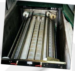
remain off until reactivated, at which point the entire cycle is repeated. The average activated operation and rest cycles of the filter are dependent on the amount of impurities flowing into the filter, the properties they contain and the condition of the filter cloth.
